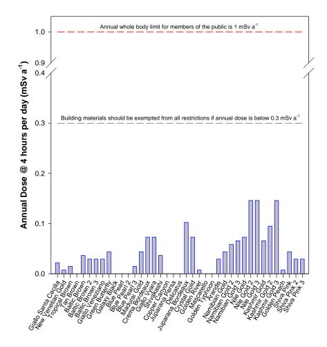
Figure 1 Annual dose (mSv a<sup>-1</sup>) from gamma radiation for each variety of stone based on the median dose measured 6 inches from the surface of the slab and assuming that the full body of a person is parallel to the slab 4 hours per day for 365 days per year. Stone types are presented in order of decreasing market share.
